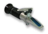
Brix is checked using a refractometer & should be performed before priming & any time syrups have been changed
